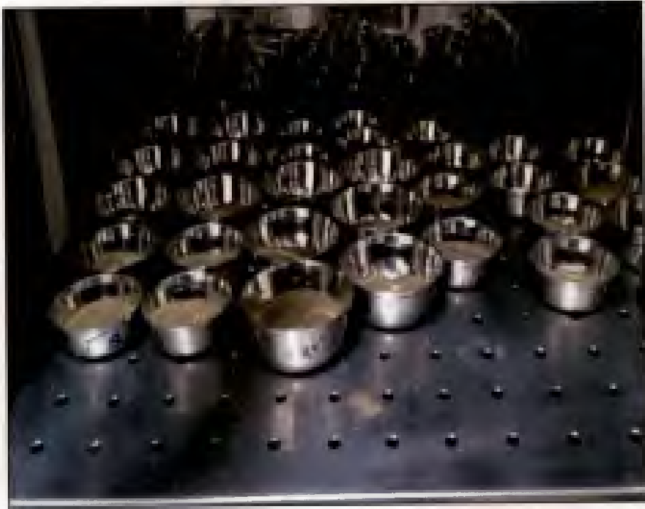
Plate 2. Soil aggregates in incubator for thermal stability studies
