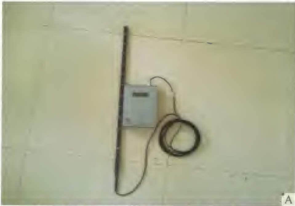
Plate 4. Photosynthetically Active Radiation (PAR) measurement in 20-year-old Acacia mangium subjected to stand thinning at Thiruvazhamkunnu, Kerala, India
