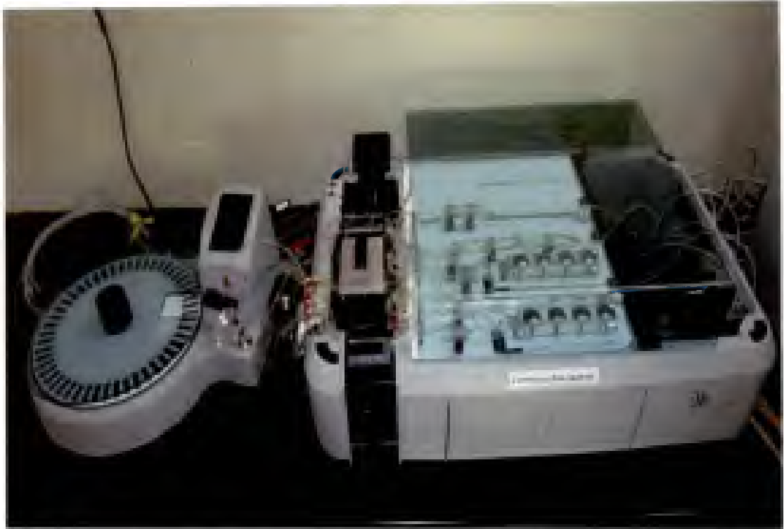
Determination of Nitrogen and Phosphorus using Continuous flow analyser
