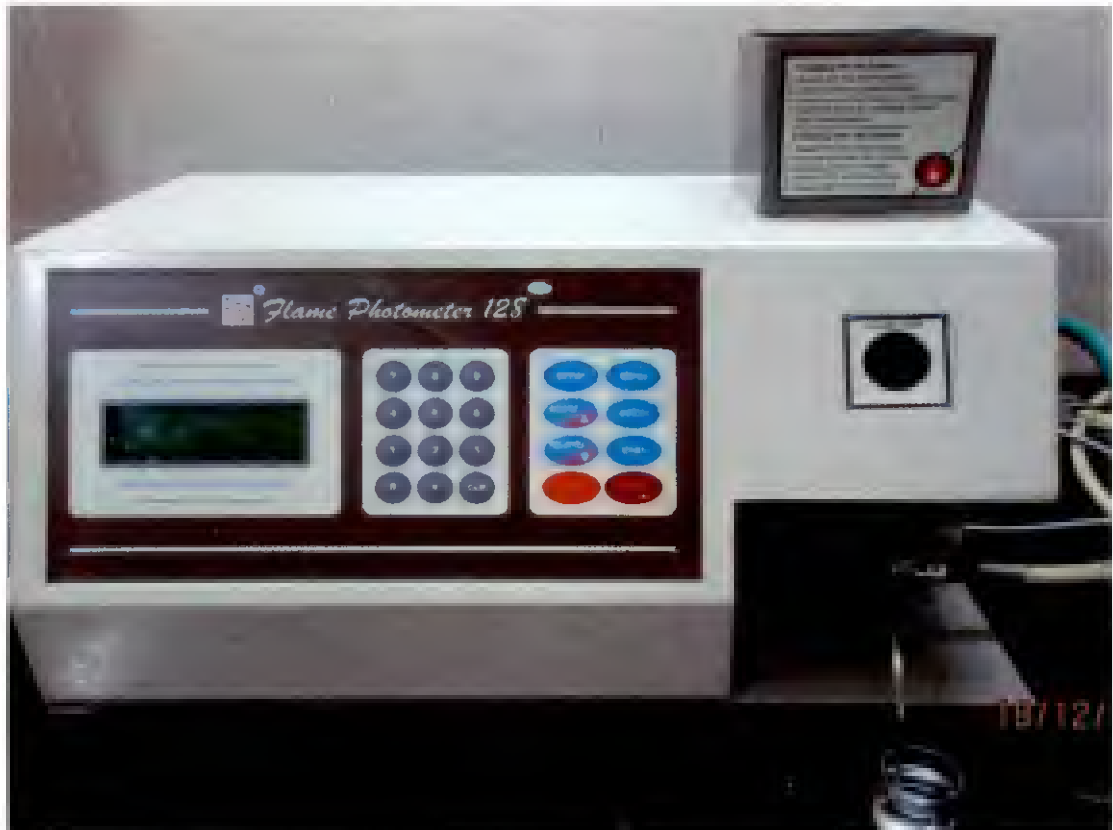
Determination of Potassium using flame photometer
