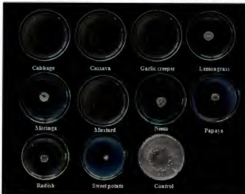
Plate 20. Effect of soil biofumigation with selected plants in confined containers on mycelial regeneration from sclerotia of R. solani (after one month)
