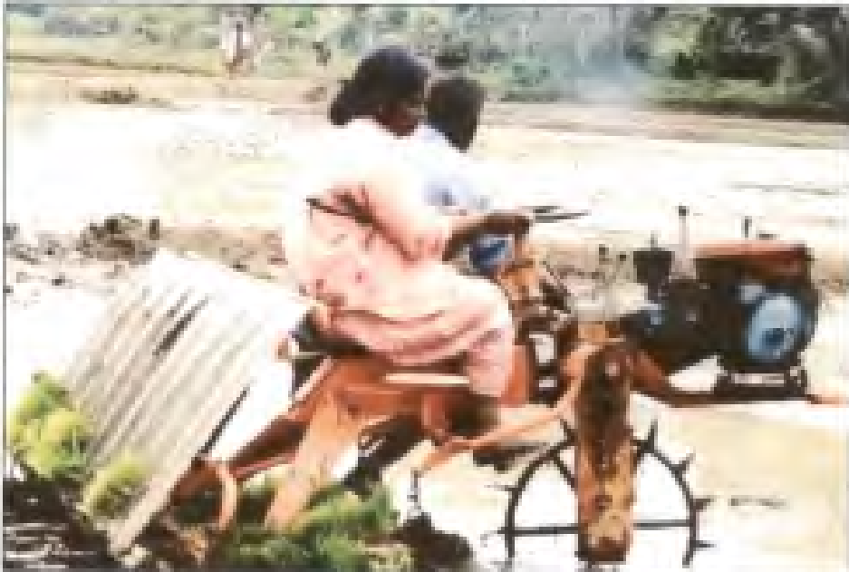
Plate 3.18 Sitting posture adopted by operator in Yanji 8 Row Self-Propelled Riding Type Rice Transplanter
