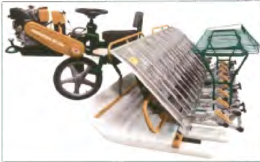
Plate 3.2 Redlands 8 row self-propelled riding type rice transplanter
