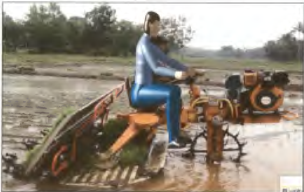
Plate 4.2 Human model posture attained by an operator in Redlands rice transplanter (posture 2)
