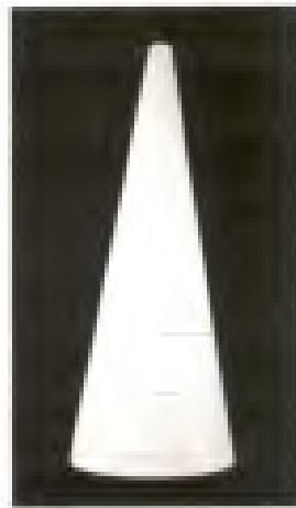
Plate 3.6 Conical device for measuring internal grip diameter
