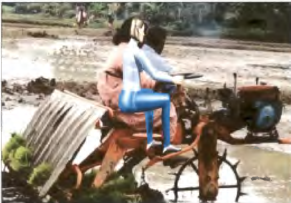
Plate 4.4 Human model posture attained by an operator in Yanji rice transplanter (posture 4)
