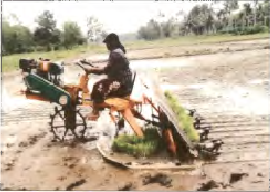
Plate 3.17 Sitting posture adopted by operator in Redlands 8 row riding type self propelled rice transplanter
