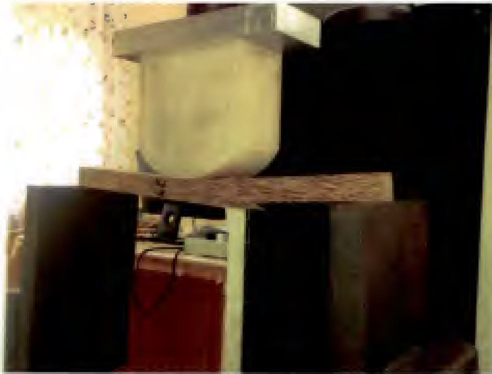
Static bending test
