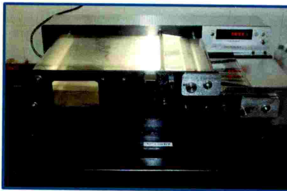
Plate 3. Leaf area meter (Model LI 3100 LI-Cor, Nebraska, USA) for measuring leaf area.
