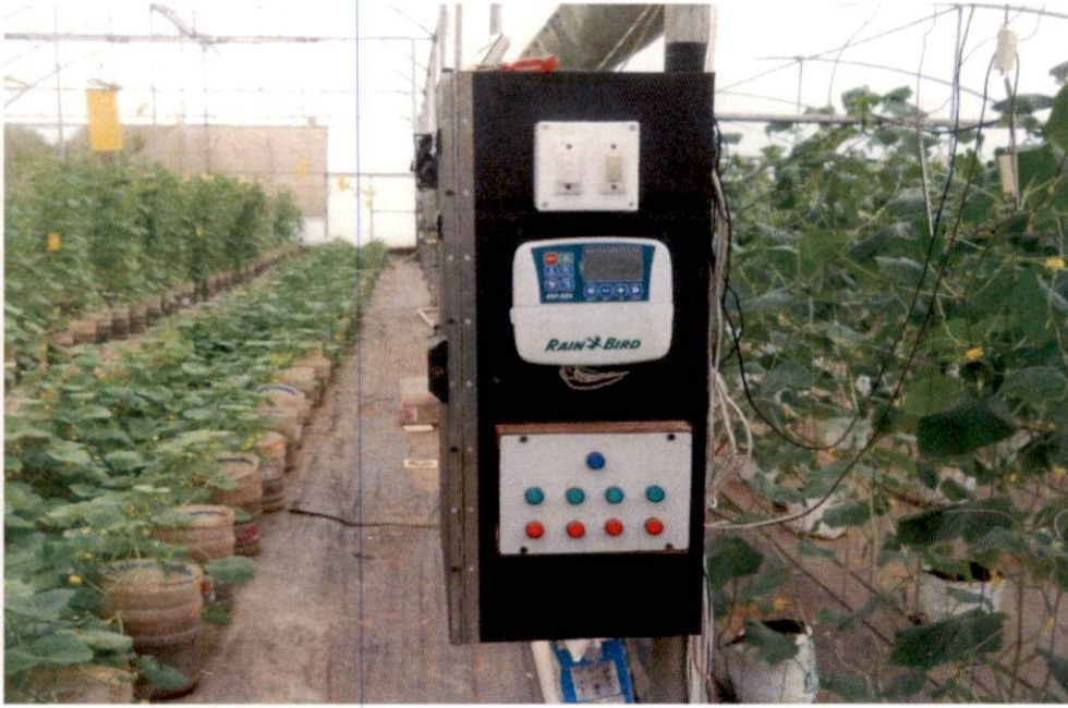
Plate 3. Side view of the wooden casing containing logical circuits
