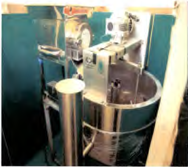
Plate 1. Machine for thermochemical digest preparation (Suchitha)
