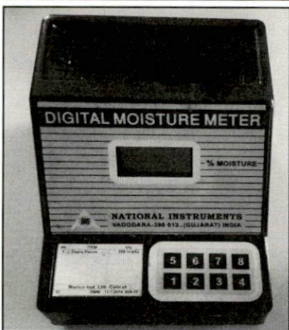
Figure 5 : Digital moisture meter used for checking the raw materials
