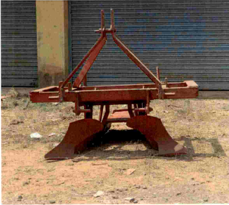
Plate 4.8 Bund strengthening implement – Model BF2
