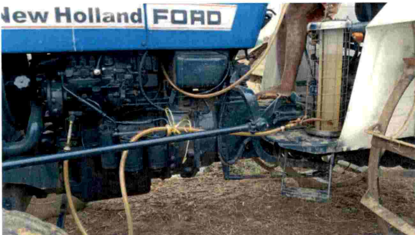
Plate 3.16 Setup for measurement of fuel consumption
