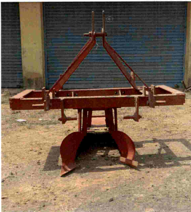
Plate 4.7 Bund strengthening implement – Model BF1
