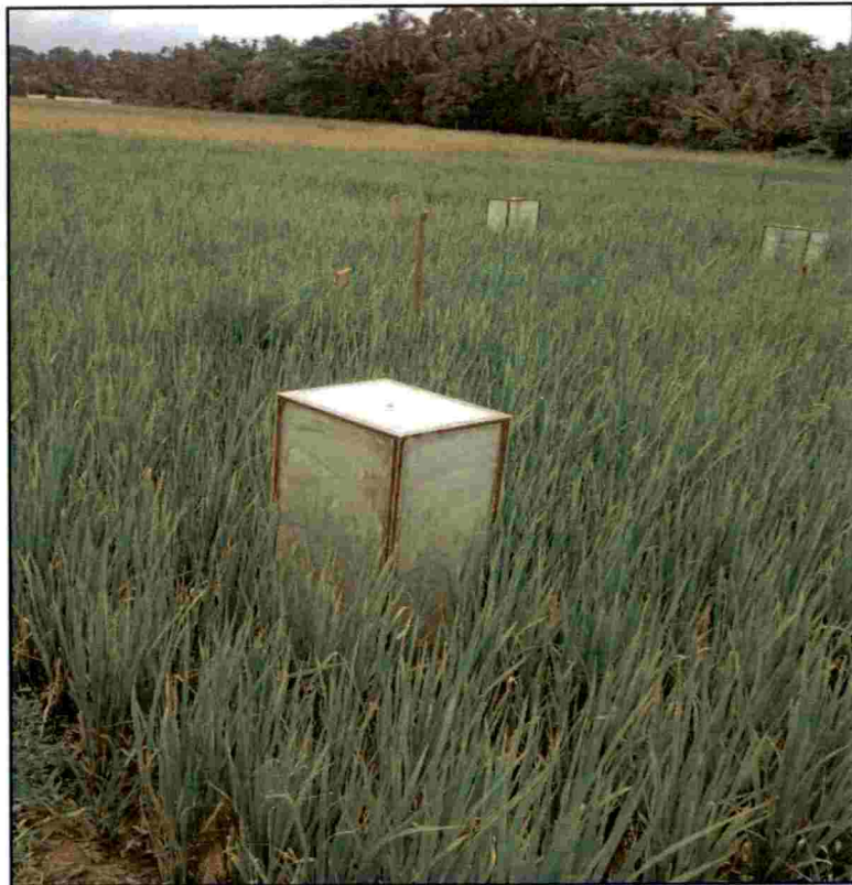
Plate 6. Box chamber with hills placed in the field for GHG collection
