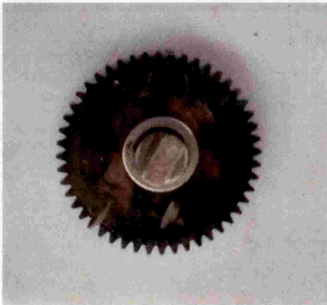
Plate.4.9. Gear with 48 teeth
