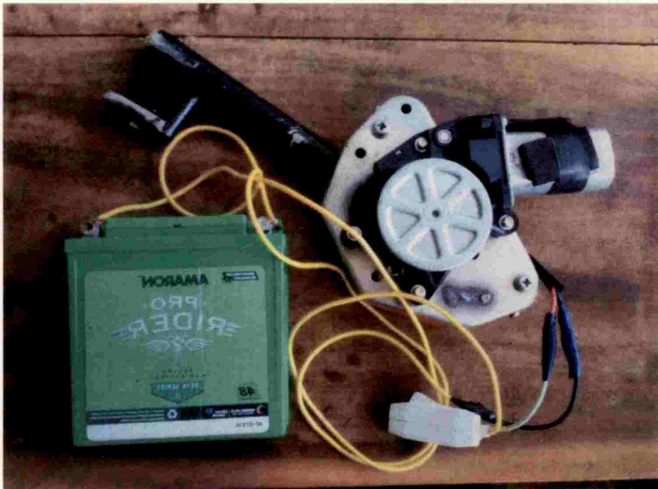
Plate.4.1. Rubber tapping machine with power source
