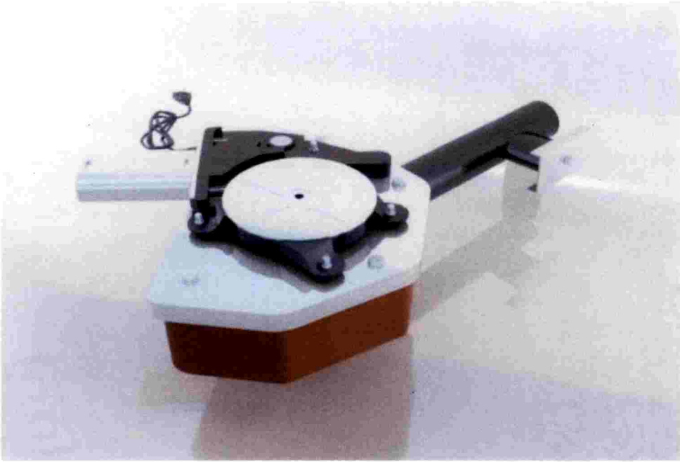
Fig.4.9 Isometric view of the rubber tapping machine
