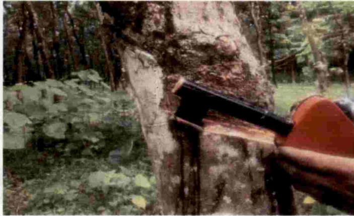
Plate.4.15. Field evaluation of rubber tapping machine
