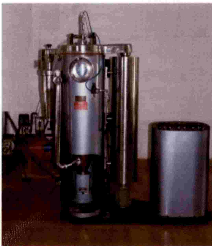
Plate 3.4 Spray dryer used for the production of microencapsulated cumin oil powder
