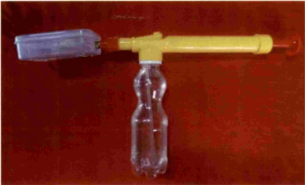
Plate 4.8 Assembled view of water assisted artificial pollinizer Model –II
