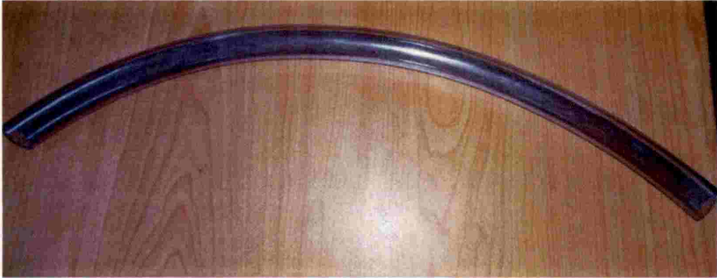
Plate 3.10 Air tube connecting chamber and vacuum pump
