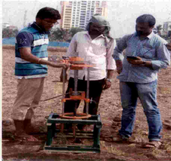
Plate 3.1 In-situ measurement of shear strength
