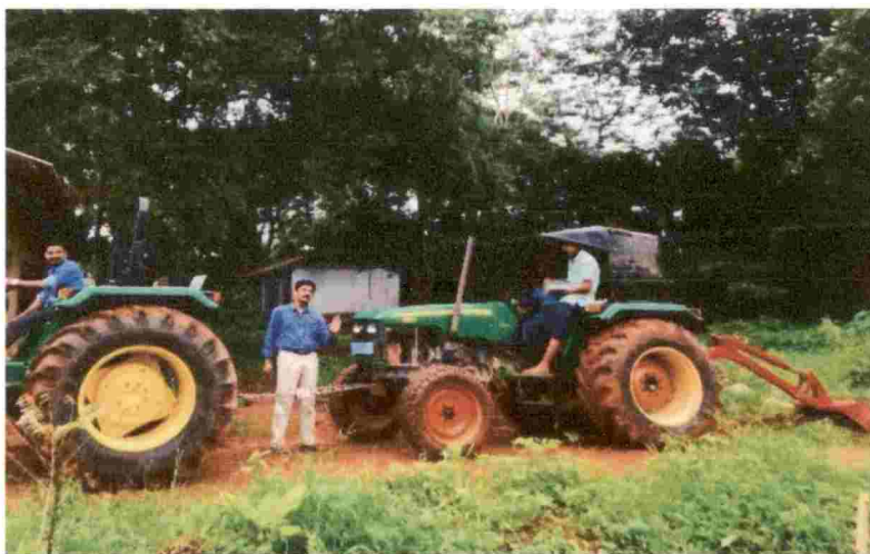
Plate 3.8 Draft measurement of the modified uprooting machine
