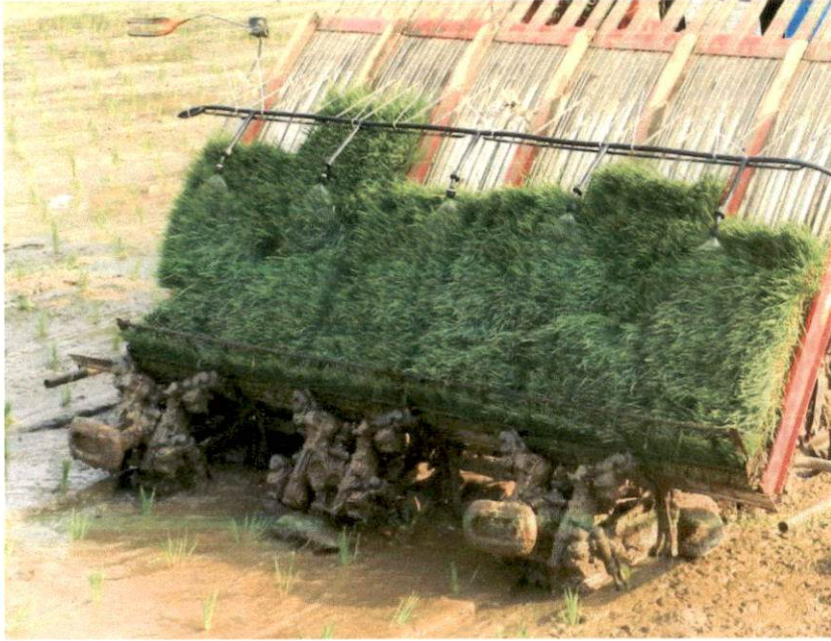
Figure 4.15 Applicator attachment fitted on the transplanter
