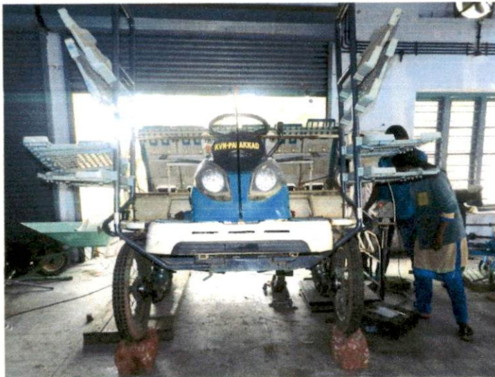
Figure 3.5 Experimental setup for finding centre of gravity
