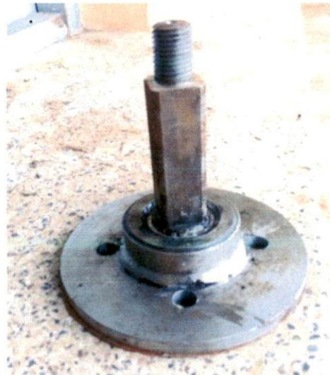
Figure 4.7 Fabricated front wheel hub attachment
