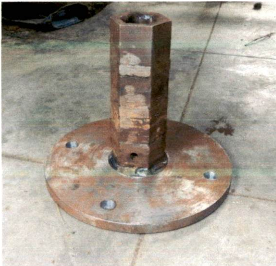
Figure 4.6 Fabricated rear wheel hub attachment
