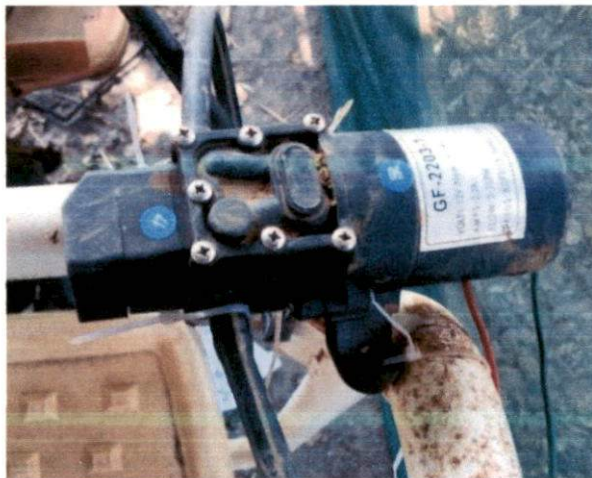
Figure 4.9 Battery operated 12 V pump
