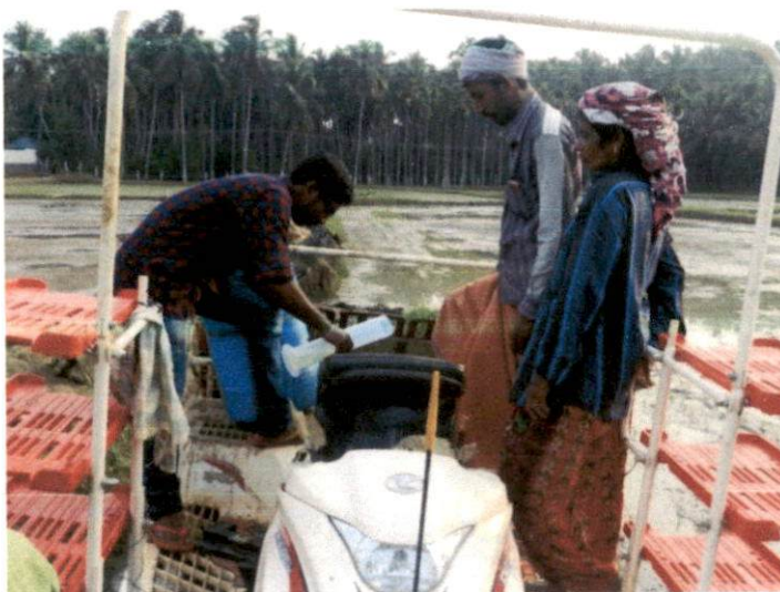
Figure 3.1 Measurement of fuel consumption
