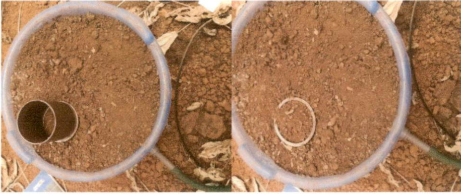
Plate 3.1 Determination of Bulk density by Core cutter
