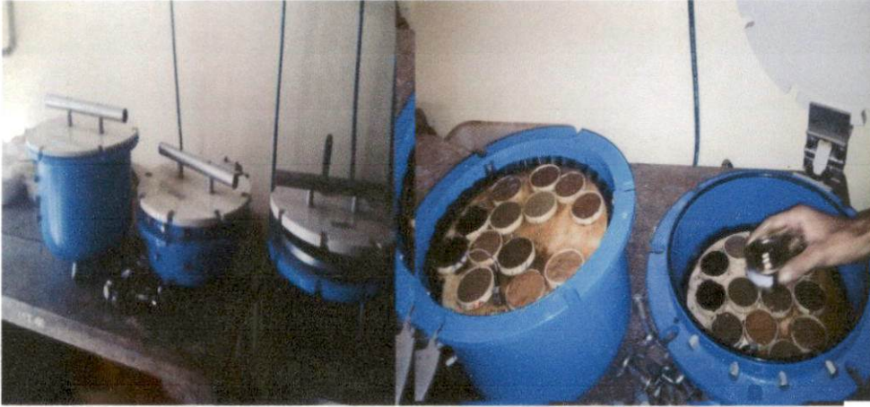
Plate 3.2 Soil moisture constants by Pressure plate apparatus
