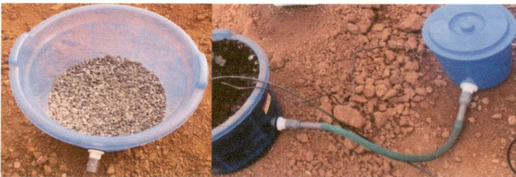
Plate 3.5 Non-weighing Mini lysimeter with drainage system
