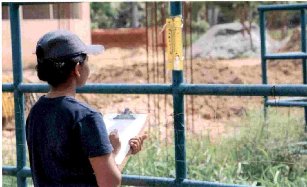
Plate 3.1 (b): Wet and Dry bulb temperature recording
