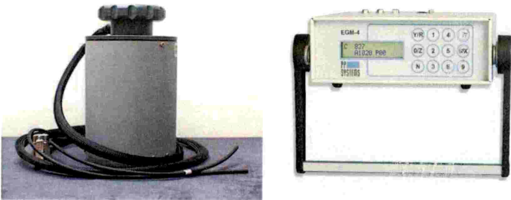
Fig 7. Soil CO 2 efflux analyzer (EGM-4) to quantify CO 2 flux from soil
