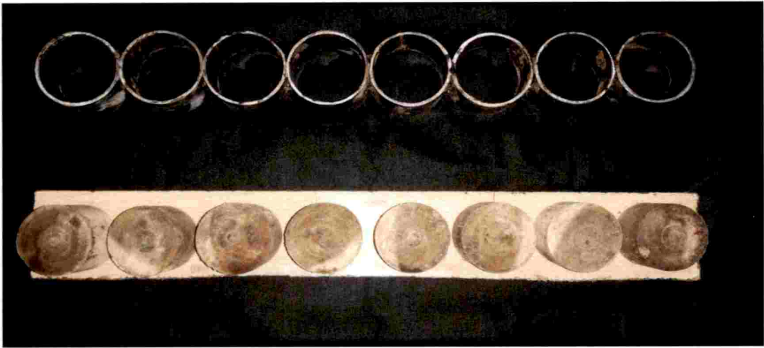
Plate 2. Mould used for the development of disc shaped matrix
