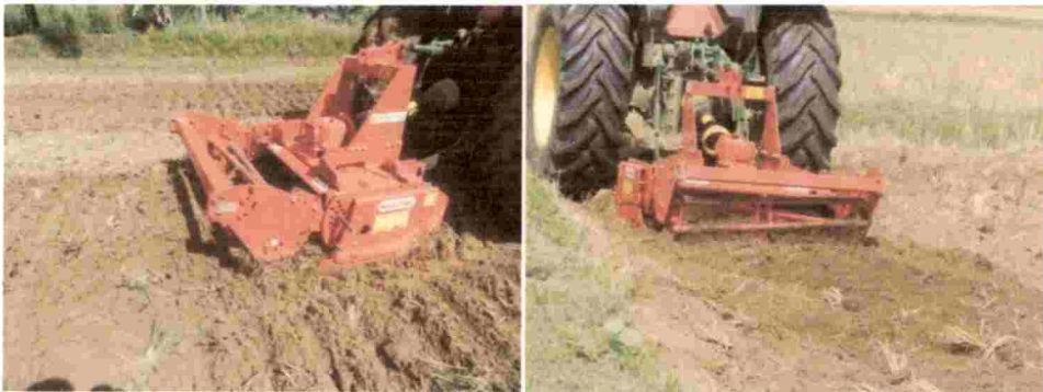
Fig. 3.8 Power harrow operation
