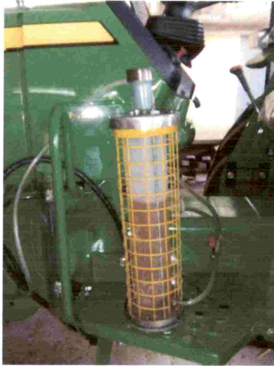
Fig. 3.6 Fuel consumption measuring setup
