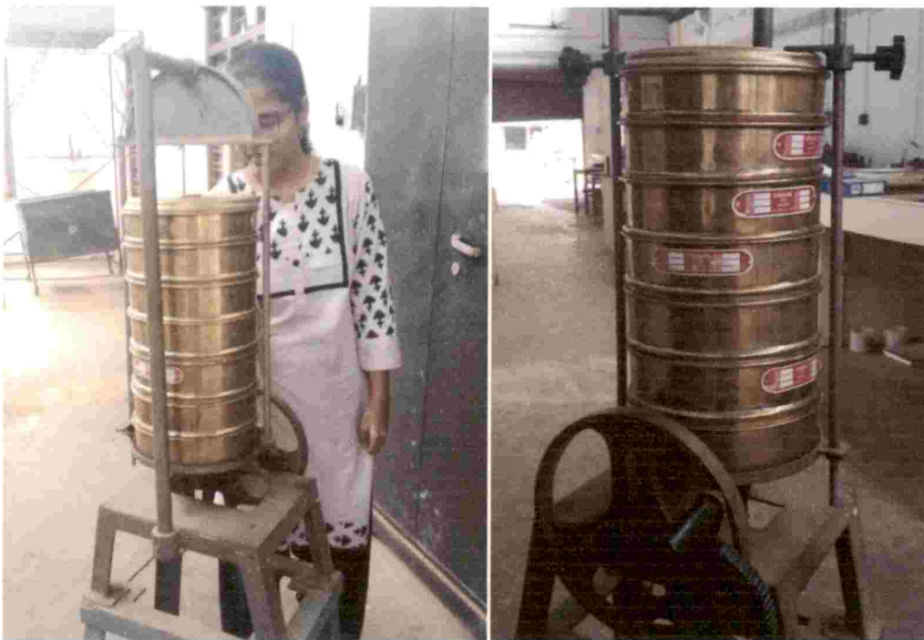
Fig. 3.5 Determination of MMD using sieve analysis
