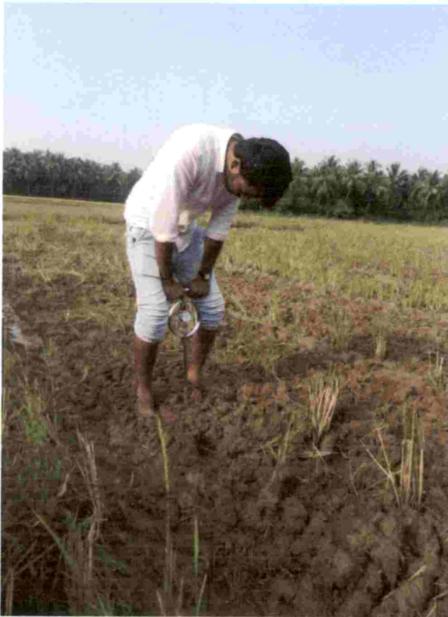
Fig. 3.3 Measurement of penetration resistance using cone penetrometer
