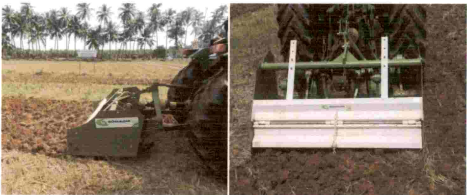
Fig. 3.9 Spading machine operation
