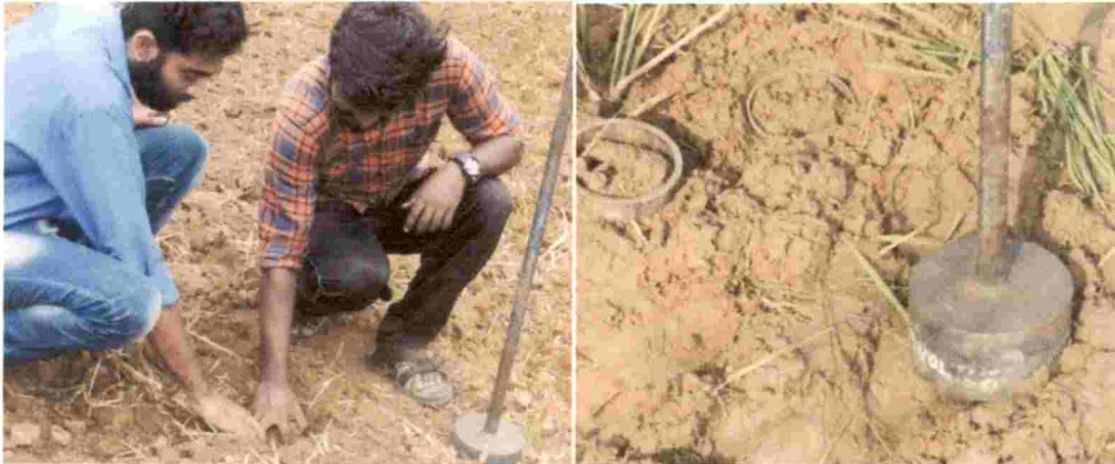
Fig. 3.2 Determination of soil bulk density by core cutter method
