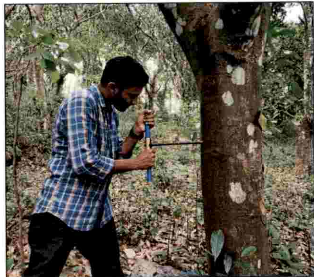
Plate 5. Collection of wood samples using Increment borer
