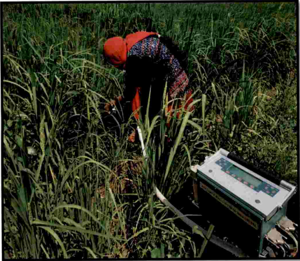
Plate. 3. Measurement of gas exchange parameters using IRGA
