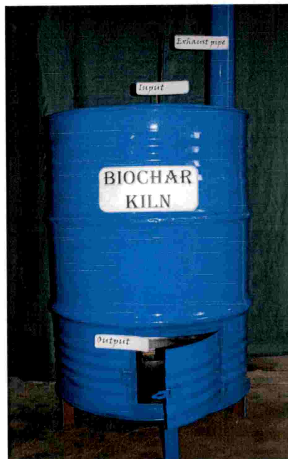
Plate 1. A view of kiln used for the production of biochar
