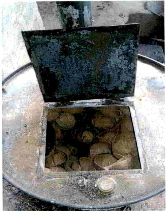
Plate 3. Filling the drum with raw material
