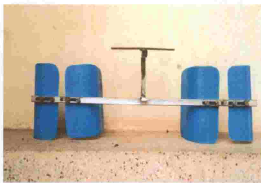
Figure 4.12 Plastic guards fixed with GI frame
