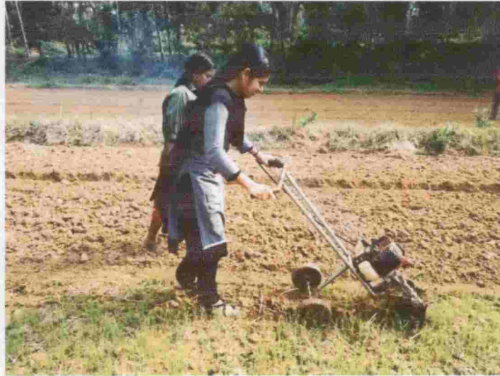
Figure 4.27 Field testing of vegetable garden weeder
