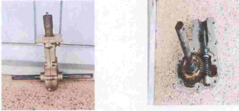
Figure 4.2 Power transmission gear box
