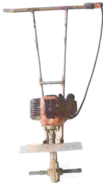
Figure 4.6 Engine mounted multipurpose tool carrier frame fitted with gear reduction unit
