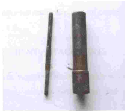
Figure 4.5 Power transmission shaft with hollow casing
