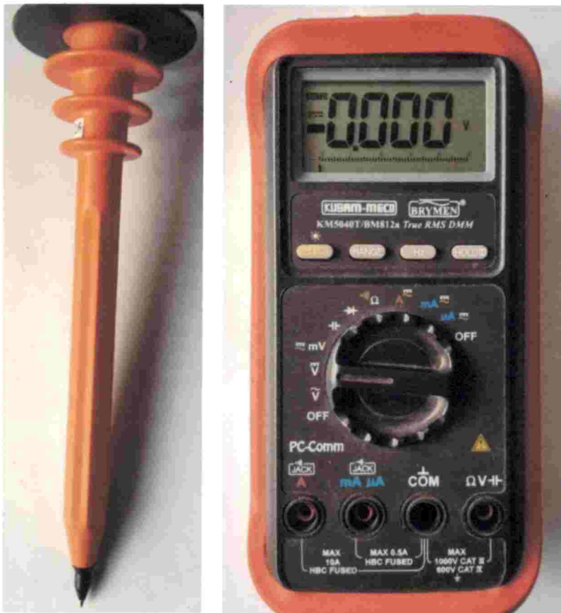
Fig. 3.12. High voltage probe and digital multi-meter
