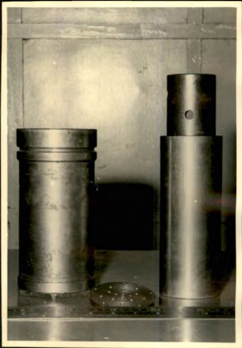
Plate no. 9 An automobile wet liner used as extraction unit, filter plate and the piston
