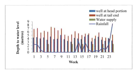
Figure 21. Depth to water table for wells along Anappara branch
