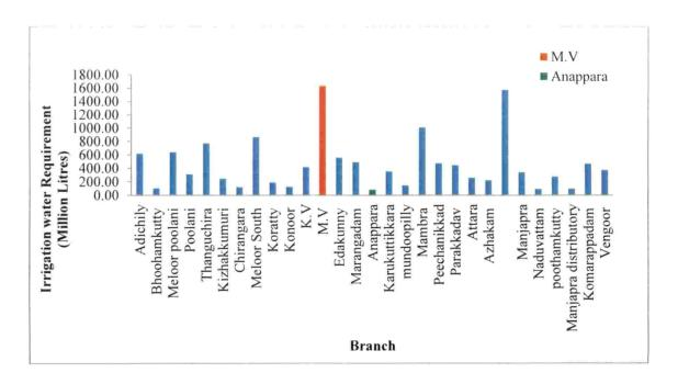
Figure 14. Total Irrigation water requirement for individual branch canal commands
