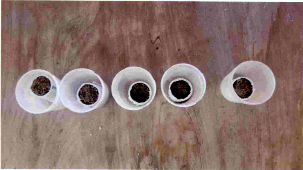
Plate 3: Cut pieces of soil column for residue analysis
