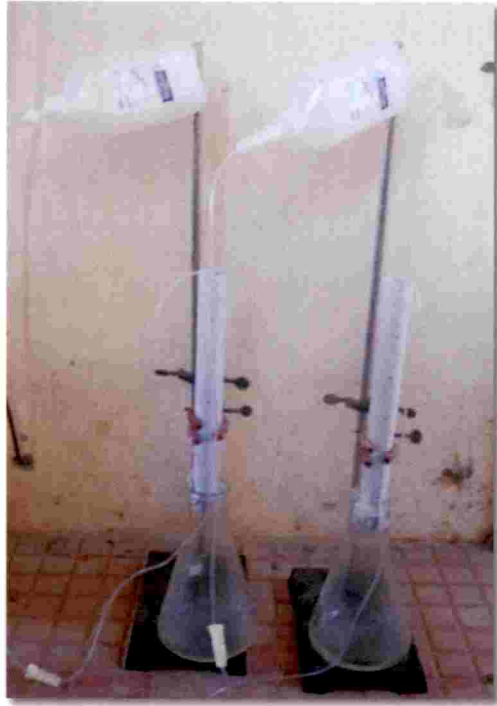
Plate 1: Elution of soil column after treatment
