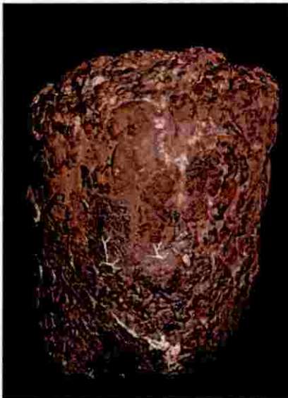
Star like crack formation phase
