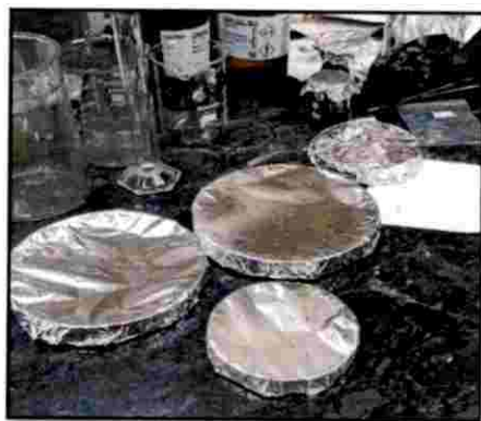
Plate 4. Films made using solvent casting method
