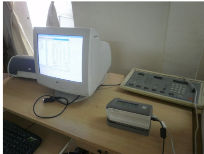
Plate 3. Spectrophotometer assembly for colour measurement
