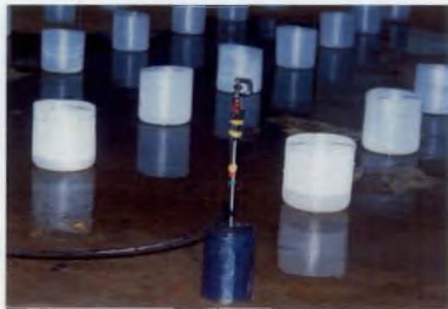
Operational Test-Emitter and catch-cans
