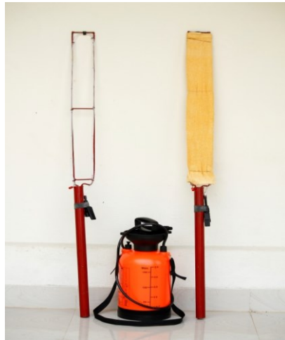
A. Wiper device developed for managing weedy rice by DCA
