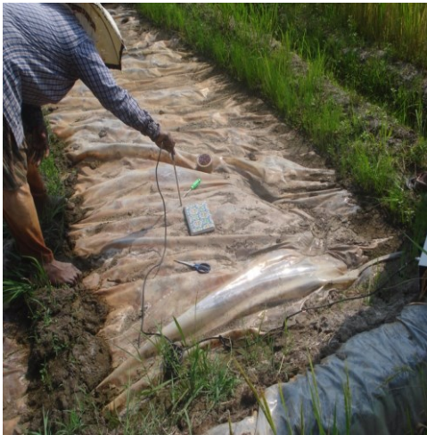
B. Measuring temperature using portable sensor
