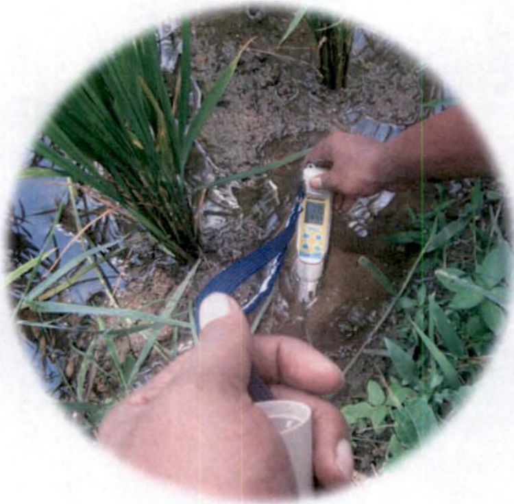
Plate 4: In-situ measurement of pH using portable pH meter
