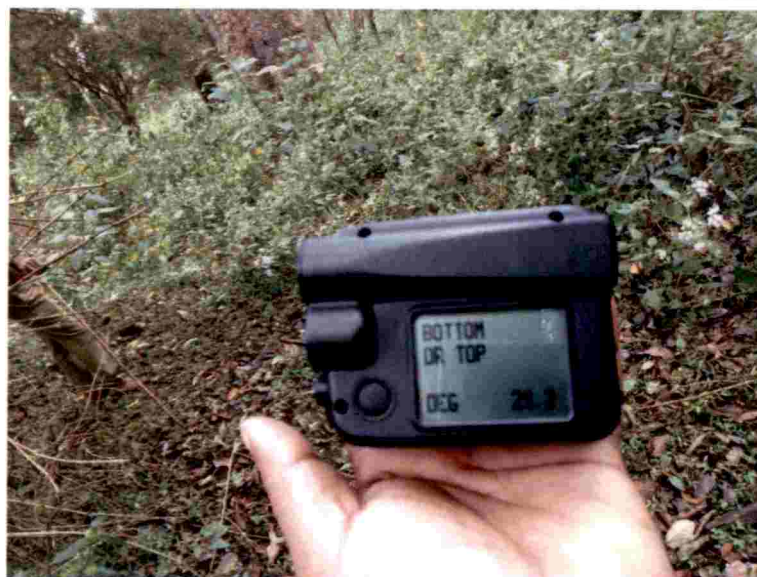
Plate 5: Vegetation studies (a) Measuring the GBH using tape; (b) Using hypsometer to measure the height
