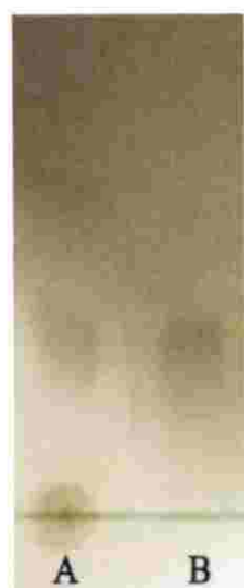
Figure 4.4: TLC plate showing re-spotted F321 fraction eluted from column chromatography of P. granatum Fruit crude hot ethanol extract shown antibacterial activity against test organisms with Rf value of 0.35 (A), Standard Ellagic acid (Rf=0.35) (B)
