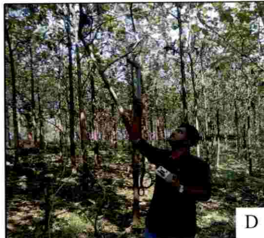
A. Measuring the height of teak trees using vertex laser hypsometer; B. Measuring girth at the breast height; C and D. Measurement of leaf area index using LAI-2000 plant canopy analyzer.
