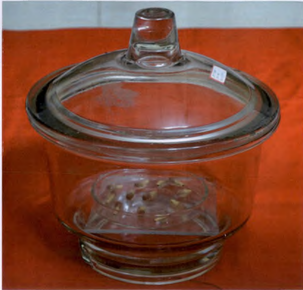
Plate 2. Desiccator with desiccation medium and synthetic cocoa seeds stored in it
