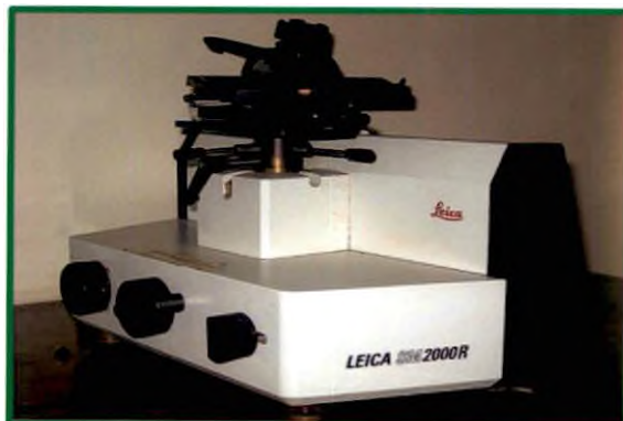
Plate 3. Sliding microtome (leica SM 2000R) used for wood sectioning
