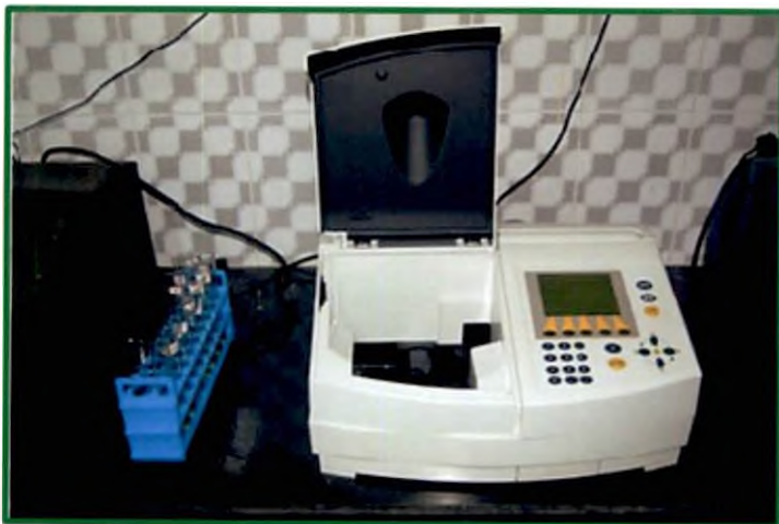
Plate 6. Spectrophotometer used for cellulose estimation
