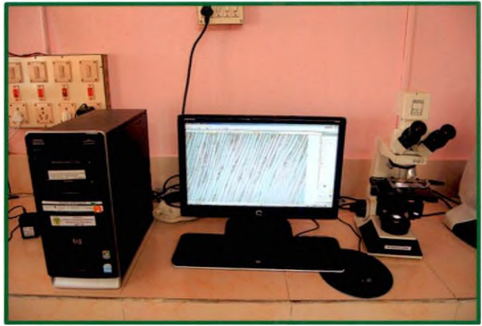
Plate 4. Image analyser (Labomed Digi-2) used for anatomical quantification
