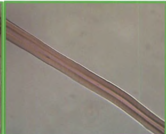
Plate 7. Photos taken using image analyser:(A) Fibre (10x) isolated by maceration, (B) Transverse section (10x) taken using sliding microtome, (C) Transverse section (40x) taken using sliding microtome, (D) Tangential section (40x) taken using sliding microtome (E) Tangential section (10x) taken using sliding microtome and (F) Fibre lumen and wall (40x) obtained by maceration
