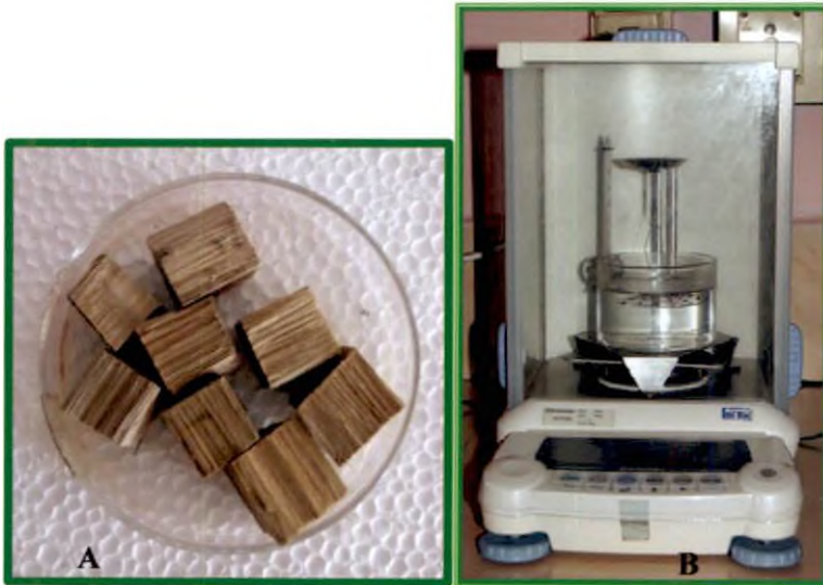
Plate 2. (A) Rectangular blocks taken from discs for specific gravity analysis, (B) Specific gravity module attached to electronic balance (Schimadzu AUY 220)
