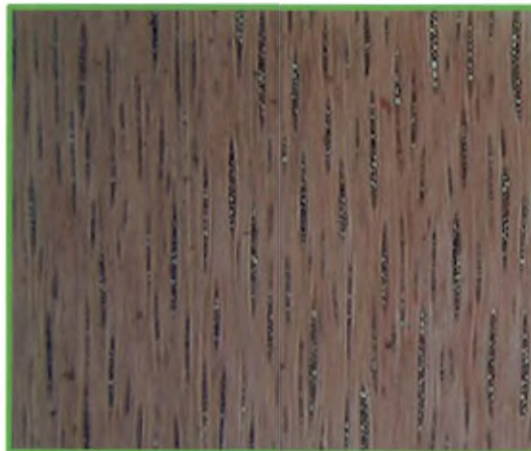
Plate 7. Photos taken using image analyser:(A) Fibre (10x) isolated by maceration, (B) Transverse section (10x) taken using sliding microtome, (C) Transverse section (40x) taken using sliding microtome, (D) Tangential section (40x) taken using sliding microtome (E) Tangential section (10x) taken using sliding microtome and (F) Fibre lumen and wall (40x) obtained by maceration
