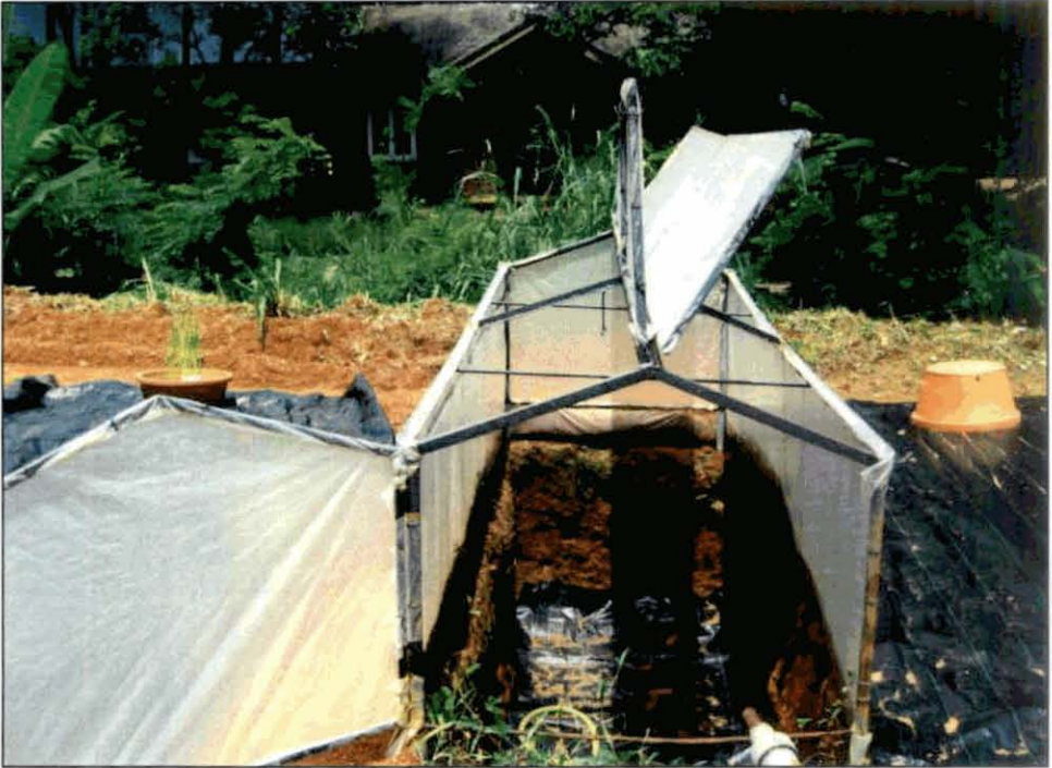
Plate 3. View of opened CO 2 trapping trench
