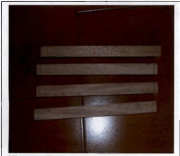
Plate 14. Scantlings (6 cm x 6 cm cross section) of nedun tree
