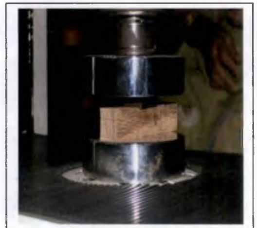
Plate 29. Test for compression strength perpendicular to grain
