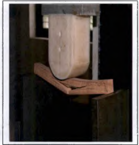
Plate 27. Static bending test
