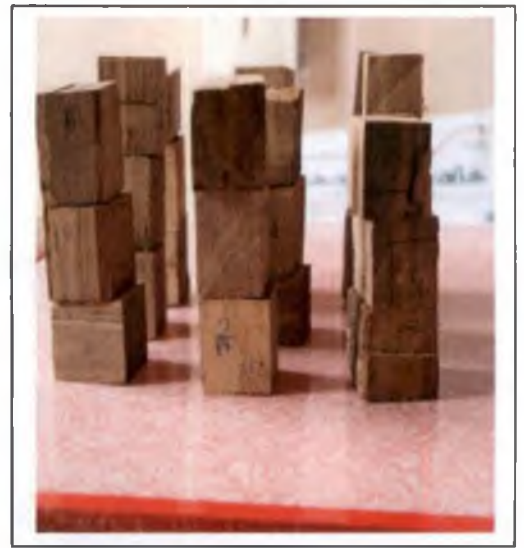
Plate 17. Wooden blocks (3cm x 3 cm x 3 cm) of nedun tree used for specific gravity analysis
