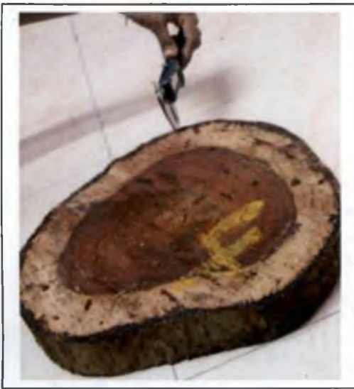
Plate 16. Measurement of bark thickness using digital vernier calliper
