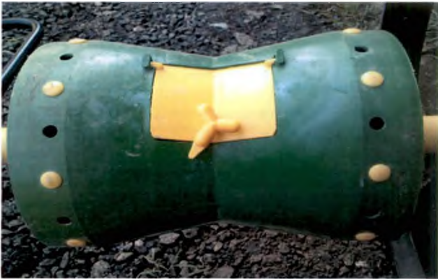
Plate 3.10 Hyperboloid shaped seed drum
