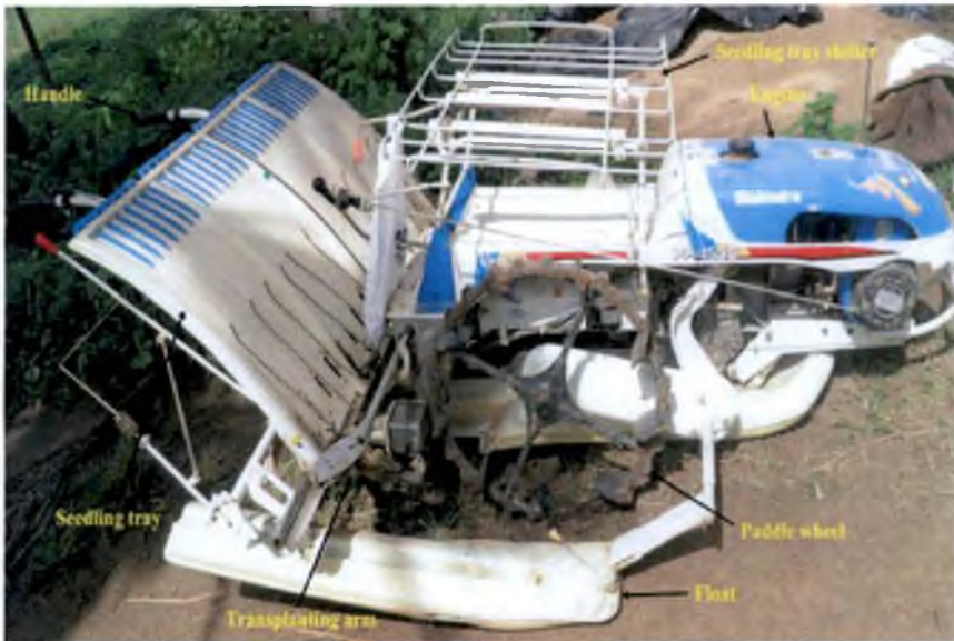
Plate 3.13 Mahindra walk behind mechanical rice transplanter
