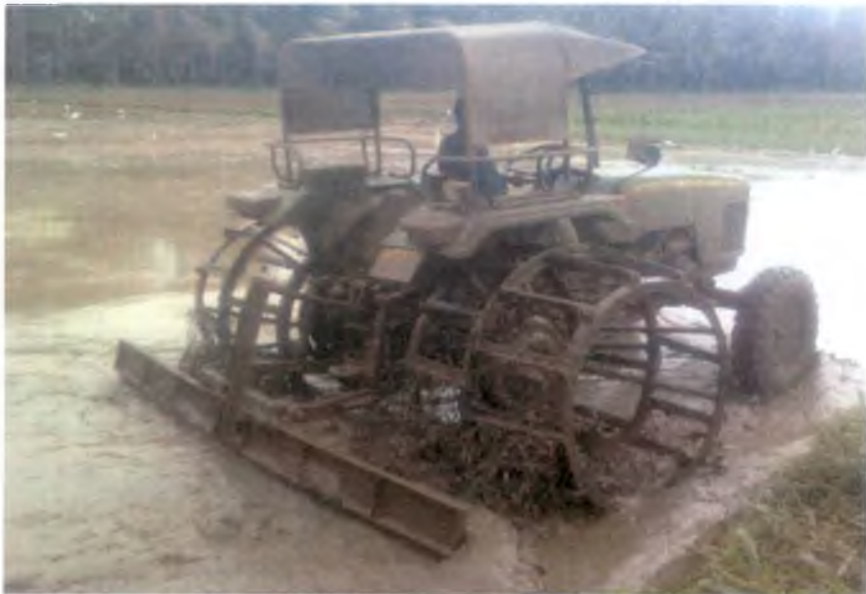
Plate 3.7 Puddling and leveling
