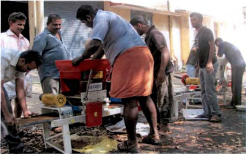
Plate 3.3 Nursery preparation using nursery raising machine
