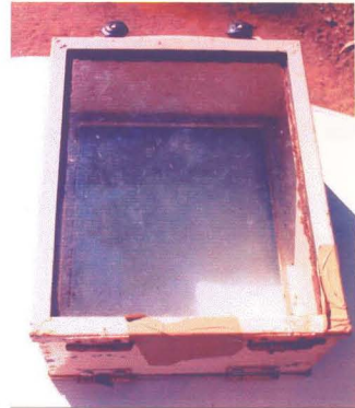
Plate 2. Leaf chamber fabricated for tracer studies
