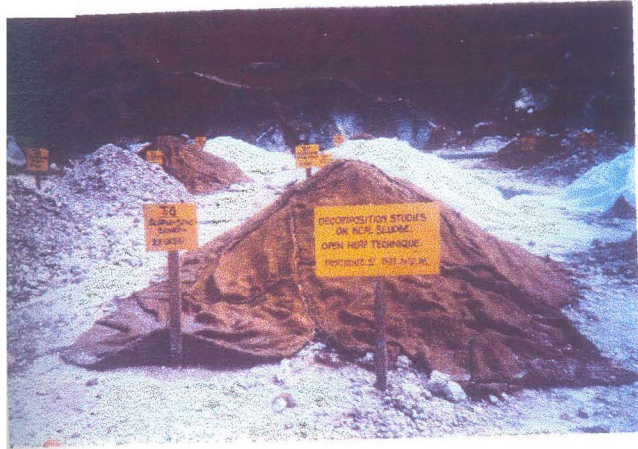
Plate 12 Aerobic open heap composting technique
