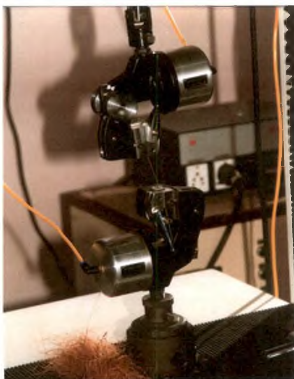
b. Banana fibre placed for testing
