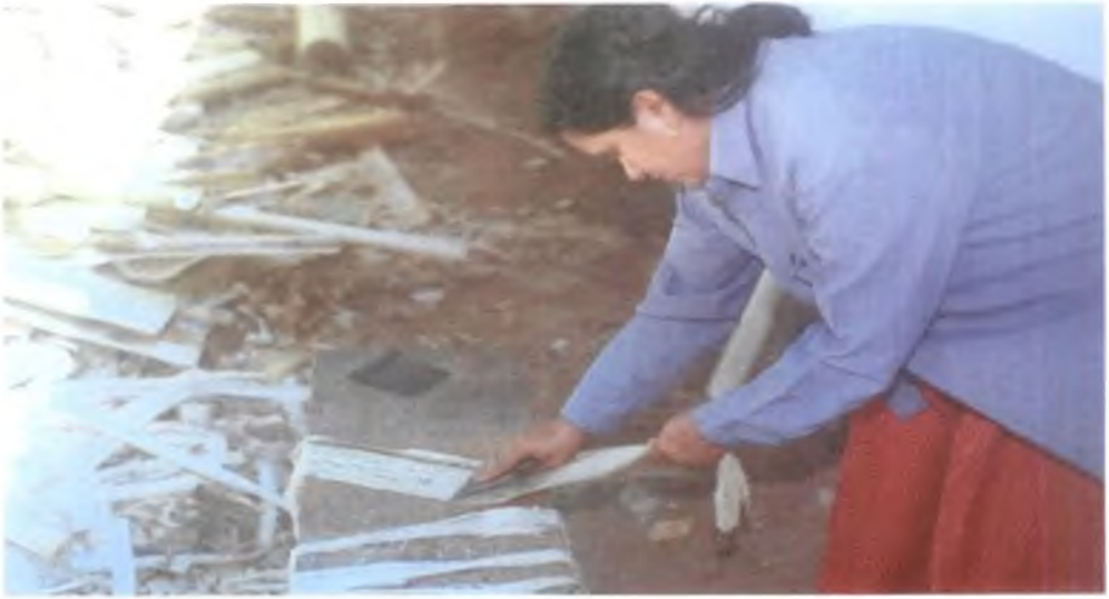
Plate 3. Extraction of banana fibre by manual method
