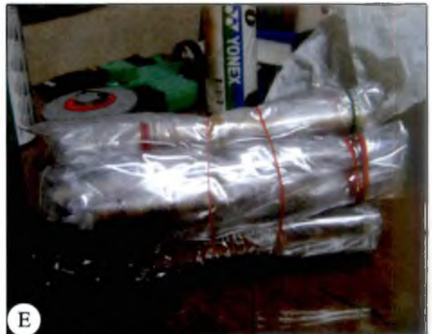
Plate 1. Collection of increment core samples of wood using Haglof increment borer CO1512: (A) Driving in the borer and inserting borer bit, (B and C) Core samples collected, (D and E) Core samples packed to prevent moisture loss
