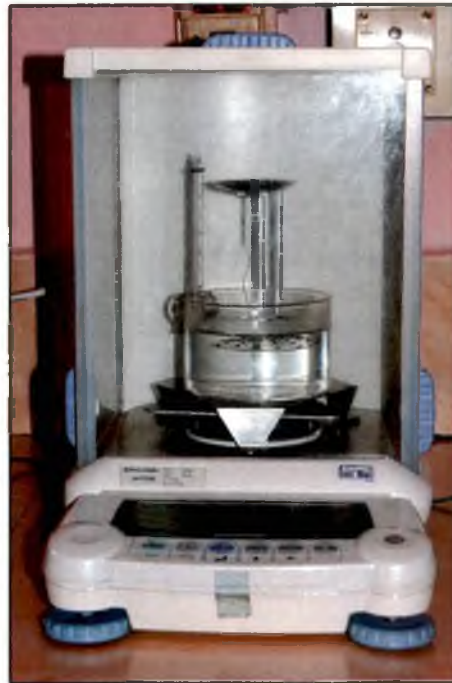
Plate 3. Specific gravity module attached to electronic balance (Schimadzu AUY 220)
