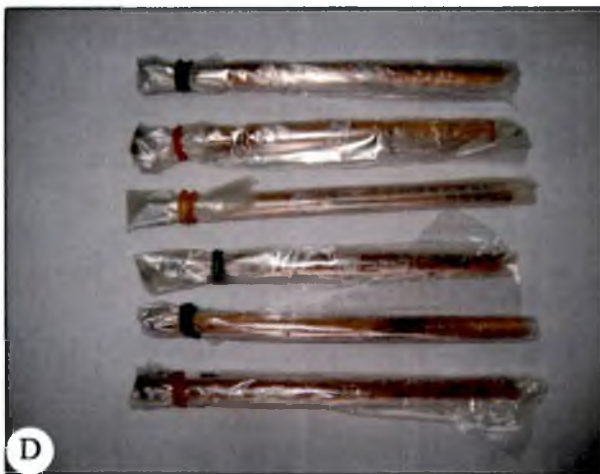
Plate 1. Collection of increment core samples of wood using Haglof increment borer CO1512: (A) Driving in the borer and inserting borer bit, (B and C) Core samples collected, (D and E) Core samples packed to prevent moisture loss
