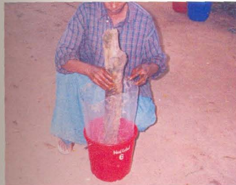
③ Compacting after adding each layer
